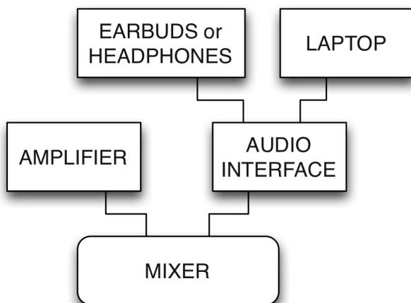
*Monitors, speakers, laptop, audio interface, and microphones are connected by cables to the mixer, which is usually placed in the back of the auditorium or on the side of the stage. Additional technical information and suggestions may be found on the TIGHT SQUEEZE page at [www.alexshapiro.org](http://www.alexshapiro.org).*
